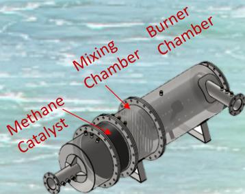
methane oxidation should also be initiated by adding heat using the fuel available for the engine. Three catalysts have been studied in a catalytic converter installed behind an 200 kW industrial lean-burn gas engine. Light-off curves and degeneration behaviour of the catalysts have been studied under real exhaust gas conditions and compositions.
